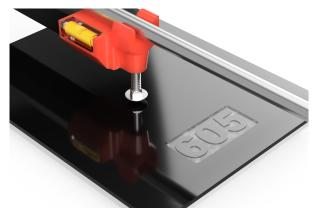
6. Use the chart below to equate the measured grams to a swingweight reading. In this example, 605 grams is equal to "D0" swingweight. If your gram reading falls in between readings on this chart, use the swingweight which is closest to your gram reading.
